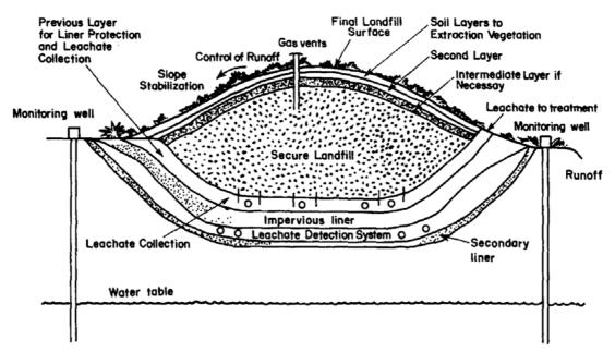
Figure (6.2) Schematic cross-section of a landfill (Visvanathan, 1996)
